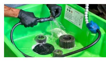
Heavy-duty cleaning for removing ink, adhesive, synthetic oils, heavy grease and other tough contaminants. These solutions work exceptionally well at room temperature and only require periodical oil skimming.
