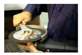
11. Always use a safety guard and make sure it is positioned properly to protect you when using the grinder.
