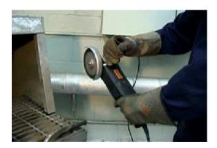
17. When using a new wheel, use less feed pressure on the first cut to "break-in" the wheel nice and round.
