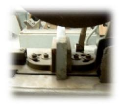
15. When cutting a work piece secured between 2 contact points, be careful that the wheel does not jam from metal piece folding down on the wheel.
