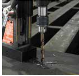
Includes a 1/2" chuck adaptor for drilling smaller holes
