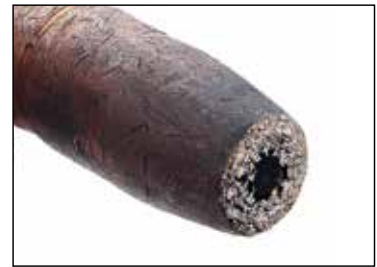
Nozzle fully clogged (not using E-WELD Nozzle)
