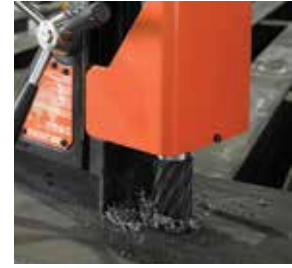
For larger holes, 1/2" and above, use the magnetic base with the standard Weldon shank
