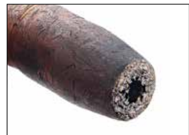
Nozzle fully clogged (not using E-WELD Nozzle)
