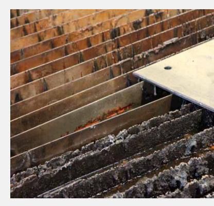
In addition to protecting tables and nozzles, ceramic heat shield solutions can also be applied to nearby areas to prevent patter and slag from sticking to exposed equipment.
