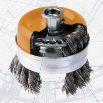
Every knot is perfectly balanced through accurate wire count and even trim length before being permanently anchored in an individual hole. This ensures perfect concentricity and vibration-free brushing for maximum operator comfort.
