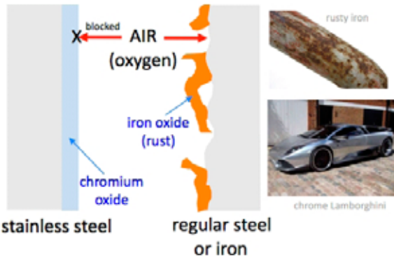
Composition of stainless steel and protective effect of the Chromium oxide layer present at the surface
