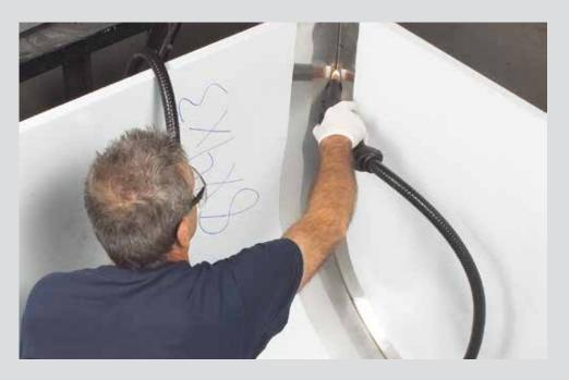
The SURFOX electrochemical weld cleaning system is a highly effective method of removing heat tint from welded stainless steel (TIG, spot, and pulsed MIG), without altering the surface of the parent material. SURFOX promotes the formation of a uniform and durable chromium oxide passive layer to protect stainless steel against further corrosion.
