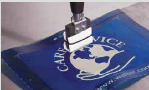
Marking with permanent stencils.
