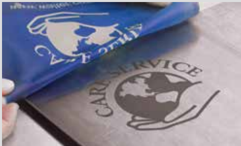
Result of black marking with permanent stencils.
