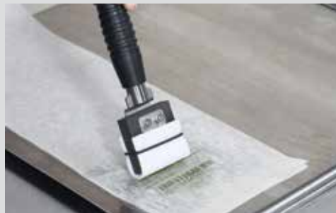
Marking with disposable stencils.
