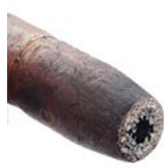
Nozzle fully clogged (not using E-WELD Nozzle)
