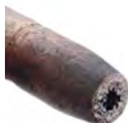
Nozzle fully clogged (not using E-WELD Nozzle)
